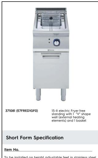
To be installed on height adjustable feet in stainless steel. High efficiency infrared heating elements (10kW) attached to the outside of the well. Deep drawn V-shaped well. Oil drains through a tap into a container under the well. Exterior panels in stainless steel with Scotch Brite finish. One piece pressed work top in 1.5 mm thick stainless steel. Rightangled side edges to allow flush-fitting junction between units.
