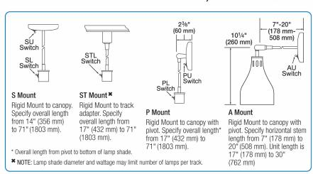
Rigid Stem Mounted (Knock down shipping on S and P units)
